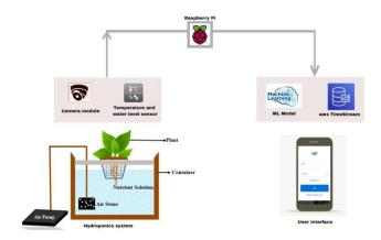
Fig. 1: Architecture of Hydroponics System
