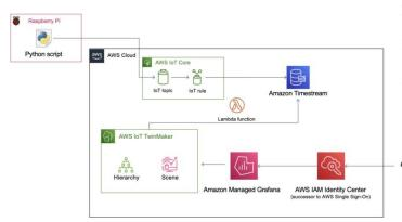
Fig. 3: Architecture of AWS TwinMaker
